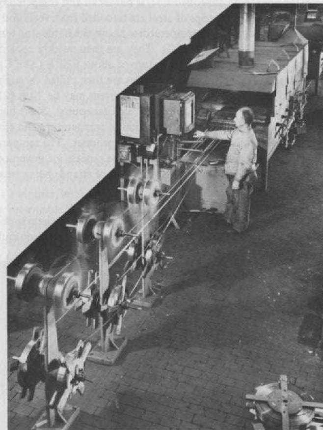
FIG. 43. Continuous hardening, quenching, and tempering six cold-rolled annealed flat strips to obtain blue tempered spring steel. (Photo courtesy American Iron and Steel Institute.)
