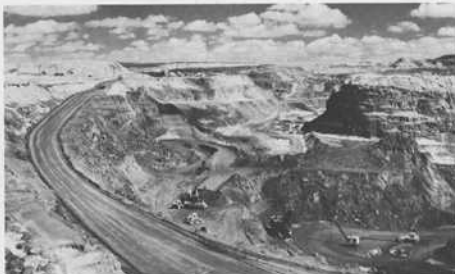
FIG. 1. Open pit iron ore mine in Minnesota, showing power shovels, trucks, and other equipment. (Photo courtesy American Iron and Steel Institute.)
