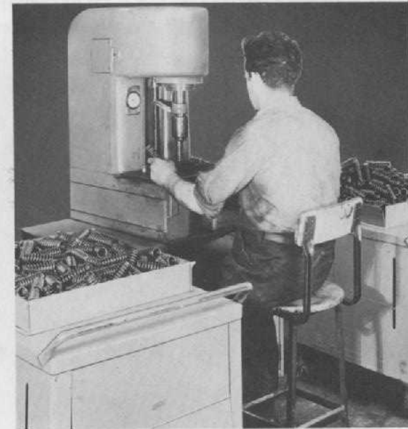
FIG. 164. Pressing springs solid to remove permanent set on a hydraulic press. Presses with turntables are often used. (Photo courtesy The Carlson Co.)
