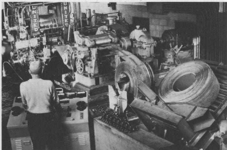
FIG. 42. Cold rolling annealed flat steel to reduce thickness of stock to desired dimensions. (Photo courtesy American Iron and Steel Institute.)
