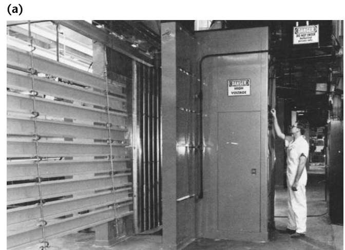
FIGURE 19. Electrostatic spray system: (a) parts enter station where electrostatic sprays apply liquid penetrant; (b) spray guns turn on only while parts move through their position.
