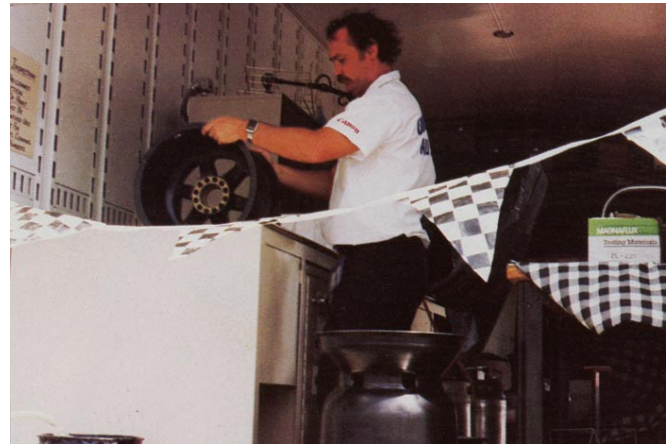
FIGURE 4. Fluorescent liquid penetrant testing of racing wheel: (a) test station; (b) indication under ultraviolet radiation.
