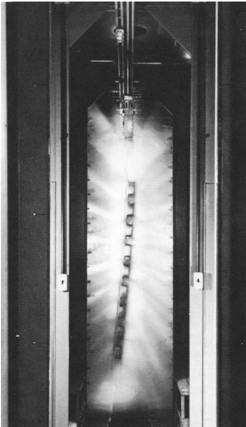
FIGURE 20. Water spray wash station for removal of surface liquid penetrant.
