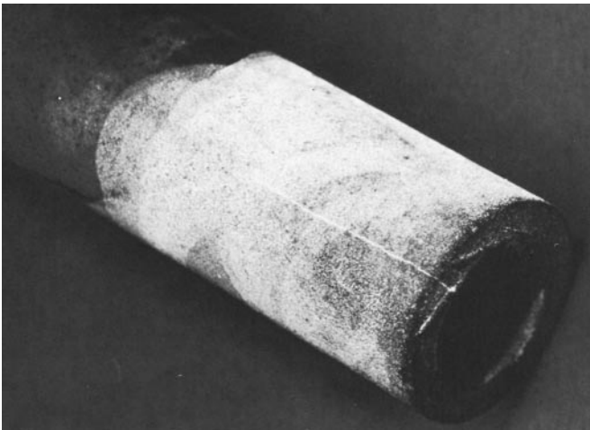
FIGURE 4. Fired, porous combustion tube with fluorescent indication of crack.
