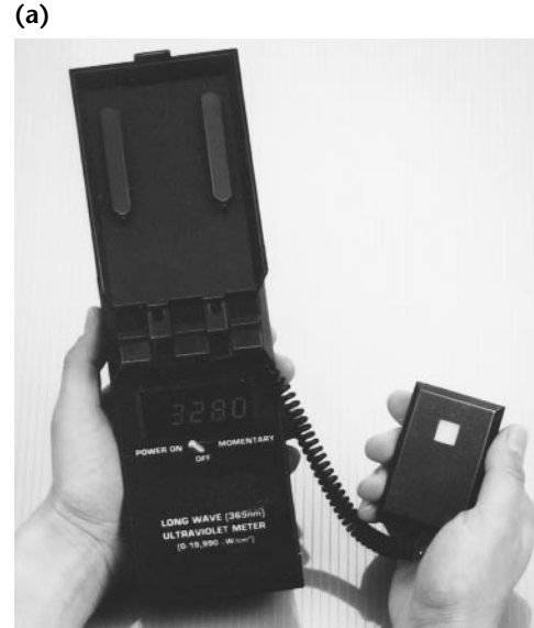
FIGURE 35. Photoelectric instruments for measurement of ultraviolet radiation intensity: (a) hand held digital ultraviolet radiometer measures near ultraviolet radiation in 0 to 19990 \mu W \cdot cm^{-2} range; (b) radiation monitoring and verification fixture ensures accurate measurement of ultraviolet radiation at 300 mm (15 in.); (c) radiometer/photometer with dual sensor for measuring ultraviolet radiation and visible (white) light.
