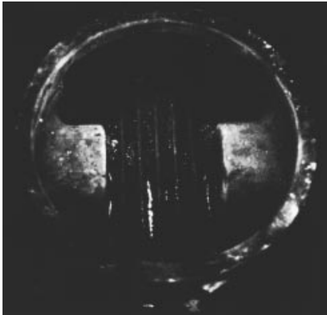
FIGURE 18. Fatigue cracks in aluminum piston head.
