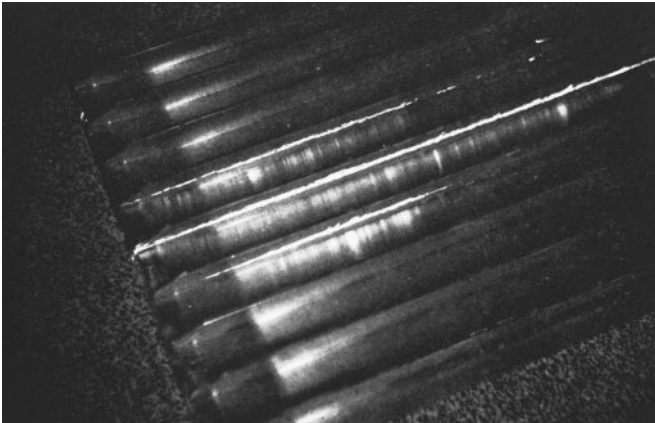
FIGURE 23. Liquid penetrant indications of discontinuities in extruded, milled, aircraft wing spar.
