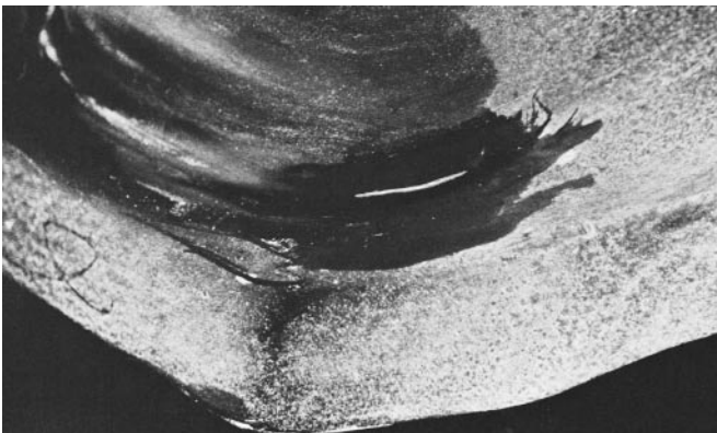
FIGURE 8. Subsurface indication of crack after removal of surface material.
