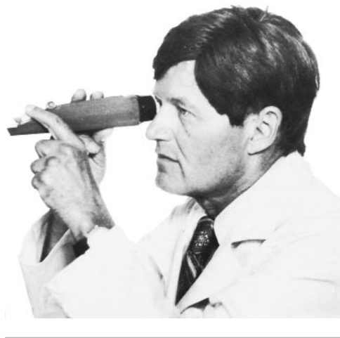
FIGURE 4. Refractometer test provides an immediate visual determination of hydrophilic emulsifier concentration.
