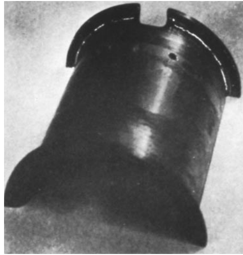
FIGURE 12. Fluorescent liquid penetrant test indications under ultraviolet radiation: (a) aluminum spar cap; (b) fatigue crack in bearing shell.
