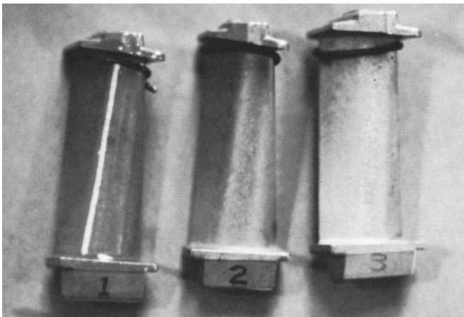
FIGURE 9. White light photograph shows three stages of prewash system: blade 1, liquid penetrant coated; blade 2, following plain water wash; and blade 3, after process completed.
