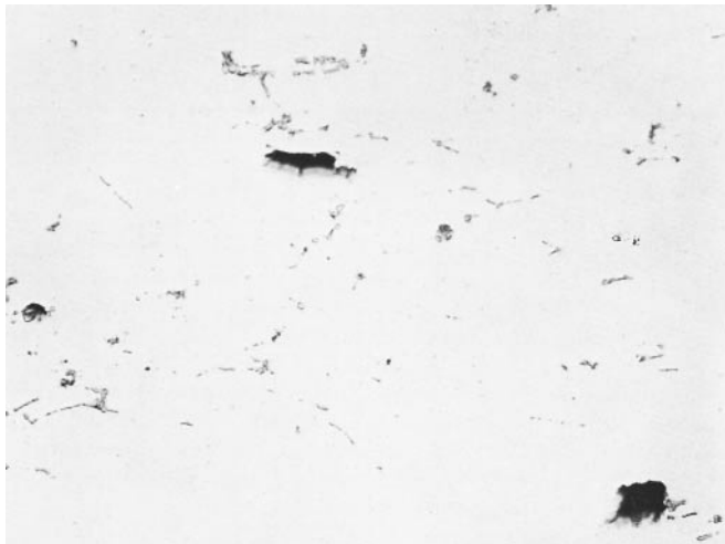
FIGURE 3. Porosity in heavy aluminum plate. Photomicrograph of pores corresponding to liquid penetrant indication near center of plate.
