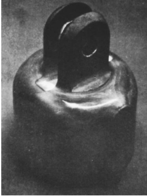
FIGURE 12. Fluorescent liquid penetrant test indications under ultraviolet radiation: (a) aluminum spar cap; (b) fatigue crack in bearing shell.
