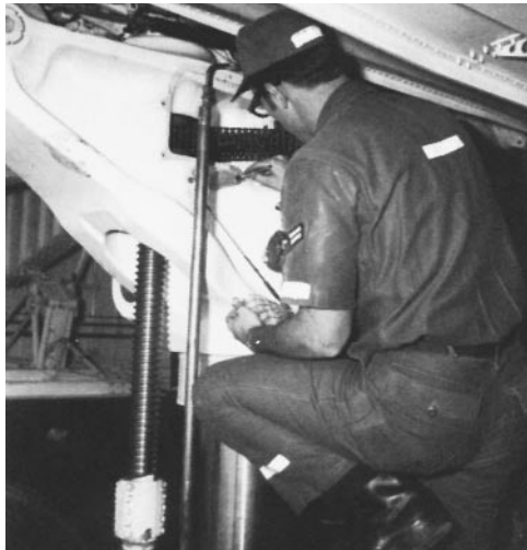
FIGURE 14. Fluorescent liquid penetrant test of landing gear forging on aircraft during maintenance operation: (a) application of liquid penetrant by brush to precleaned test area; (b) wipe removal of excess surface liquid penetrant from test area.
