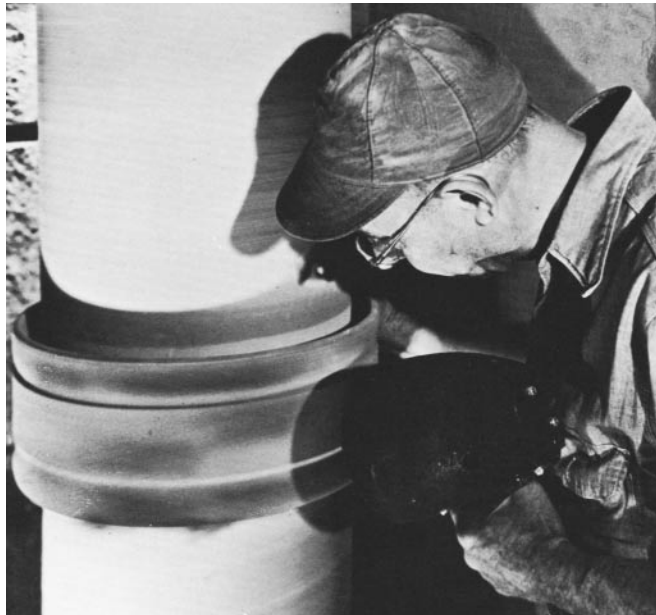
FIGURE 10. Portable ultraviolet lamp used in fluorescent inspection of high tension bushing.
