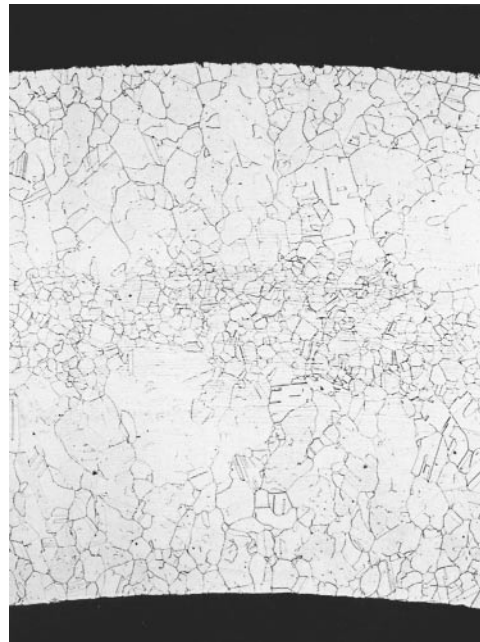
FIGURE 2. Photomicrograph of sensitized AISI 304 stainless steel specimen (typical of five control specimens not coated with liquid penetrant test materials), after 80 day stress corrosion test in warm, moist atmosphere and after oxalic acid etch: (a) sensitized specimen; (b) etched specimen.
