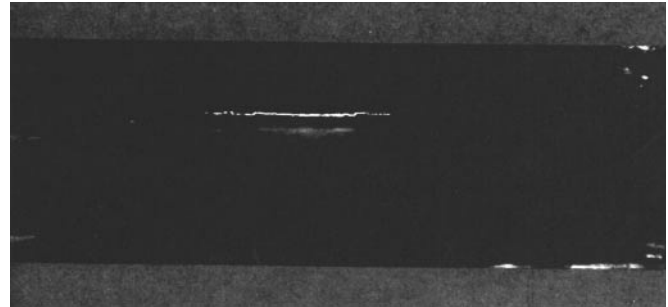
FIGURE 12. Crack in stainless steel tube: (a) fluorescent liquid penetrant indication; (b) cross section.
