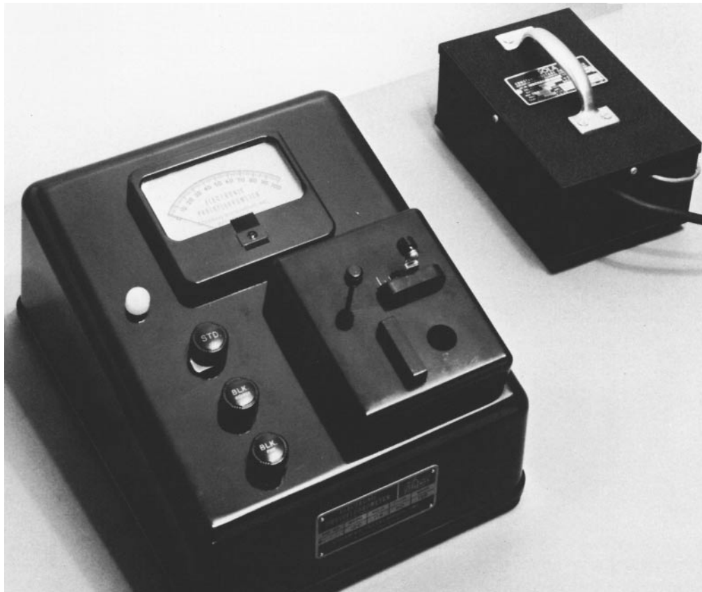
FIGURE 1. Laboratory fluorometer specified by MIL-I-25135 1 and ASTM E 1135 6 and containing built-in ultraviolet radiation source and interchangeable filters for light modification.
