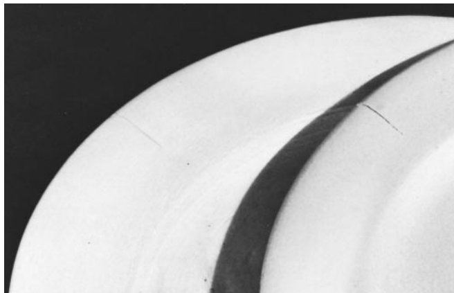
FIGURE 12. Unfired (left) and fired (right) hotel chinaware containing similar defects.
