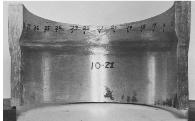
FIGURE 2. Surface defects in base metal near circumferential weld in nuclear power plant piping: (a) white light photograph of inside surface, showing weld location and contour of weld root area (note wall thickness change at weld); (b) fluorescent liquid penetrant indications in base metal, paralleling weld root area between 13 and 18 inch marks; (c) microscopic photograph of cross section through pipe wall showing nonmetallic sliver in base metal.
