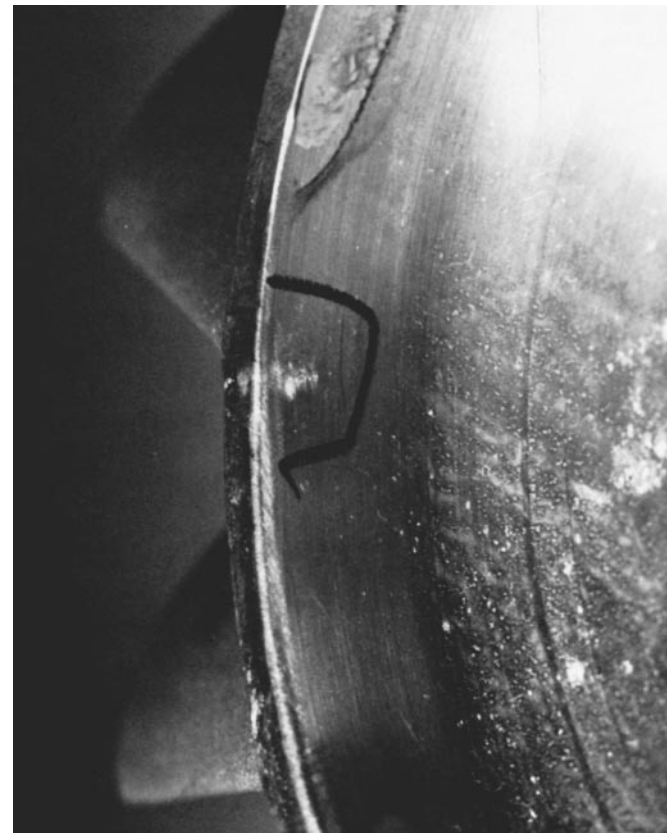
FIGURE 7. Example of working standard and interpretation guide for 356-T6 aluminum alloy casting with line of porosity that will propagate into a fatigue crack and cause failure. This condition is in stressed area, so fan casting should be rejected.
