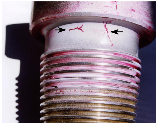
FIGURE 2. Crack indications on connection outside diameter after development time.
