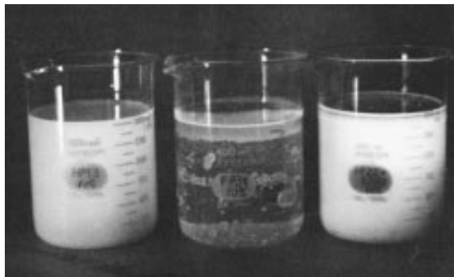
FIGURE 8. Prewash liquid penetrant effluent floats (center beaker) whereas effluents from water washable (hydrophilic) liquid penetrant (left) and postemulsifiable (lipophilic) liquid penetrant (right) form emulsions.
