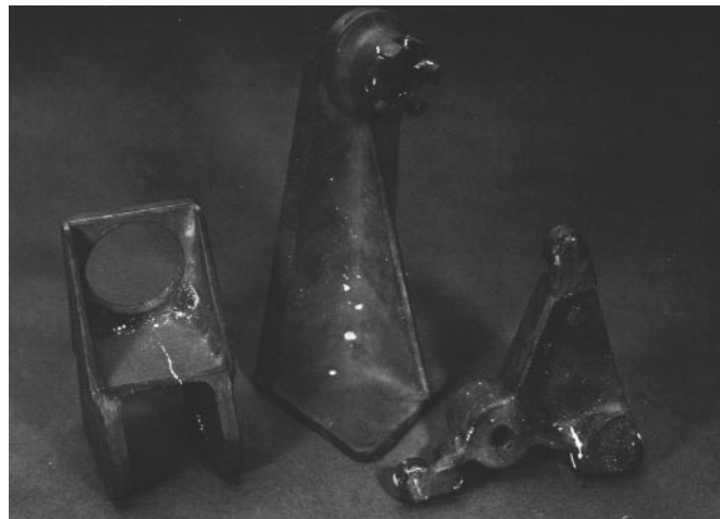
FIGURE 1. Fluorescent liquid penetrant indications of porosity and shrinkage cracking in cast light alloy aircraft fittings.
