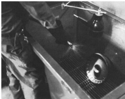
FIGURE 8. Techniques for water rinse removal of excess liquid penetrant: (a) proper use of coarse water spray at 45 degree angle to wash parts to remove water washable liquid penetrant; (b) improper adjustment of water hose nozzle for parts washing.
