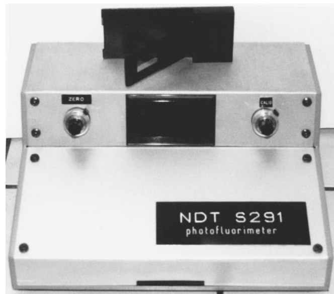
FIGURE 3. Another type of fluorometer for measuring penetrant brightness.
