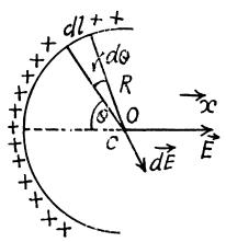
3.9 From the symmetry of the condition, it is clear that, the field along the normal will be zero
