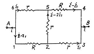
$$R_0 = \frac{\varphi_A - \varphi_B}{i} = \frac{\left[\frac{R+r}{3r+R}(r-R) + R\right]i}{i} = \frac{r(3R+r)}{3r+R}$$
