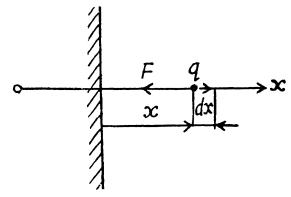
3.56 (a) Using the concept of electrical image, it is clear that the magnitude of the force acting on each charge,
