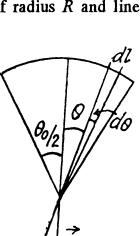
(b) Using the solution of 3.14 (a), net field strength at O due to stright parts equals  $\sqrt{2} \left( \frac{\sqrt{2} \lambda}{4 \pi \epsilon_0 R} \right) = \frac{\lambda}{2 \pi \epsilon_0 R}$  and is directed vertically down. Now using the solution of 3.15
