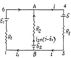
3.183 Indicate the currents in all the branches using charge conservation as shown in the figure. Applying loop rule,  $-\Delta \varphi = 0$  in the loops 1A781, 1B681 and B456B, respectively, we
