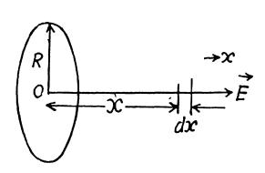
3.12 (a) The given charge distribution is shown in Fig. The symmetry of this distribution implies that vector  $\overrightarrow{E}$  at the point O is directed to the right, and its magnitude is equal to the sum of the projection onto the direction of  $\overrightarrow{E}$  of vectors  $d\overrightarrow{E}$  from elementary charges dq. The projection of vector  $d\overrightarrow{E}$  onto vector  $\overrightarrow{E}$  is
