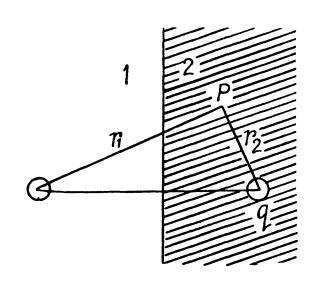
3.93 To calculate the electric field, first we note that an image charge will be needed to ensure that the electric field on the metal boundary is normal to the surface.
