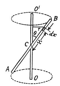
1.270 Let us consider the system in a frame rotating with the rod. In this frame, the rod is at rest and experiences not only the gravitational force  $m \ \overline{g}$  and the reaction force R, but also the centrifugal force  $F_{cf}$ .
