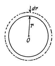
3.28 Using Gauss theorem we can easily show that the electric field strength within a uniformly charged sphere is  $\vec{E} = \left(\frac{\rho}{3 \epsilon_0}\right) \vec{r}$
