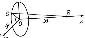
3.13 (a) It is clear from symmetry considerations that vector  $\vec{E}$  must be directed as shown in the figure. This shows the way of solving this problem: we must find the component  $dE_r$  of the field created by the element dl of the rod, having the charge dq and then integrate the result over all the elements of the rod. In this case
