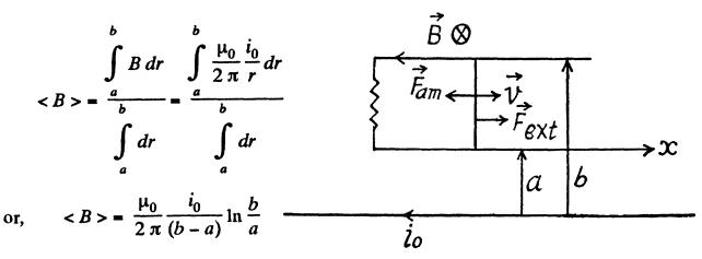
(a) The flux of  $\overrightarrow{B}$  changes through the loop due to the movement of the connector. According to Lenz's law, the current in the loop will be anticlockwise. The magnitude of motional e.m.f.,
