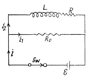
3.336 To find the magnetic field energy we recall that the flux varies linearly with current. Thus, when the flux is  $\Phi$  for current i, we can write  $\phi = A i$ . The total energy inclosed in the field, when the current is I, is
