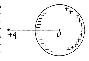
3.64 As the sphere has conducting layers, charge -q is induced on the inner surface of the sphere q and consequently charge +q is induced on the outer layer as the sphere as a whole is uncharged.
