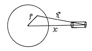
When the flux changes, an e.m.f.  $-N \frac{d\Phi}{dt}$  is induced and a current  $-\frac{N}{R} \frac{d\Phi}{dt}$  flows. The total charge q, flowing, as the magnet is removed to infinity from x = 0 is,
