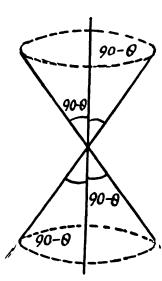
1.283 Here  $M = I \omega$  is along the symmetry axis. It has two components, the part  $I \omega \cos \theta$  is constant and the part  $M_{\perp} = I \omega \sin \theta$  presesses, then
