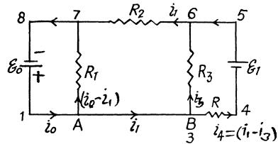
3.184 Indicate the currents in all the branches using charge conservation as shown in the figure. Applying the loop rule  $(-\Delta \varphi = 0)$  in the loops 12341 and 15781, we get
