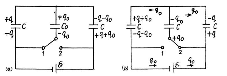
After the switch is thrown to position 2, the charges change as shown in (Fig-b).
