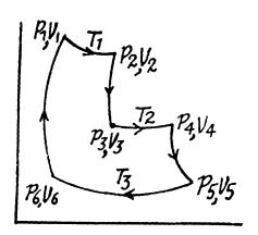
Thus  $Q_2$  = heat ejected at the lower temperature =  $-RT_3 \ln \frac{V_6}{V_5}$
