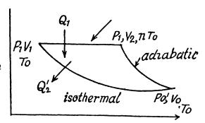
2.121 Here the isothermal process proceeds at the maximum temperature instead of at the minimum temperature of the cycle as in 2.120.
