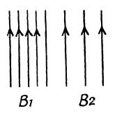
(b) Here, the external field must be  $\frac{B_1 - B_2}{2}$  upward with an internal field,  $\frac{B_1 + B_2}{2}$ , upward on the left and downward on the right. Thus,
