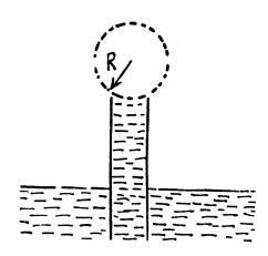
2.167 Initially the pressure of air in the capillary is  $p_0$  and it's length is l. When submerged under water, the pressure of air in the portion above water must be  $p_0 + 4\frac{\alpha}{d}$ , since the level of water inside the capillary is the same as the level outside. Thus by Boyle's law
