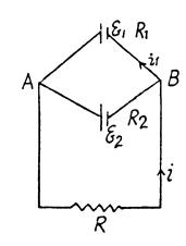
Thus one can replace the given arrangement of the cells by a single cell having the emf  $\xi_0$  and internal resistance  $R_0$ .
