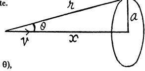
where,  $2\pi (1 - \cos \theta)$  is the solid angle, formed by the disc like surface, at the charge.
