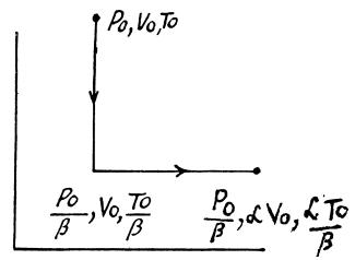
$$= (-C_V \ln \beta + C_P \ln \alpha) v = \frac{vR}{\gamma - 1} (\gamma \ln \alpha - \ln \beta) \approx -11 \frac{\text{Joule}}{{}^{\circ}K}$$
