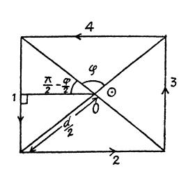
Magnetic induction due to the arc segment at O,
