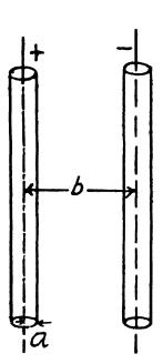
3.109 The field in the region between the conducting plane and the wire can be obtained by using an oppositely charged wire as an image on the other side.
