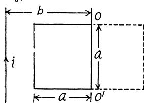
Then it can be easily seen that in the final position,  $\Phi_2 > 0$ , while in the initial position,  $\Phi_1 < 0$  (the normal is opposite to  $\overline{B}$ ), and  $\Delta \Phi$  turns out to be simply equal to the fulx through the surface bounded by the final and initial positions of the frame:
