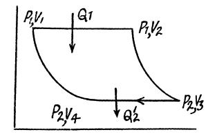
2.119 Since the absolute temperature of the gas rises n times both in the isochoric heating and in the isobaric expansion
