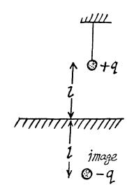
3.55 By definition, the work of this force done upon an elementry displacement dx (Fig.) is given by
