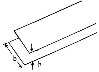
3.322 For a single current carrying wire,  $B_{\varphi} = \frac{\mu_0 I}{2\pi r} (r > a)$ . For the double line cable, with current, flowing in opposite directions, in the two conductors,
