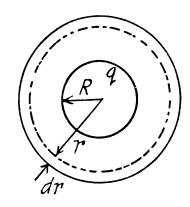
3.27 Let us consider a spherical layer of radius r and thickness dr, having its centre coinciding with the centre of the system. Then using Gauss' theorem for this surface,
