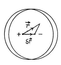
The electric field  $\overrightarrow{E_0}$  in a spherical cavity in a uniform dielectric of permittivity  $\varepsilon$  is related to the far away field  $\vec{E}$ , in the following manner. Imagine the cavity to be filled up with the dielectric. Then there will be a uniform field E everywhere and a polarization P, given by,
