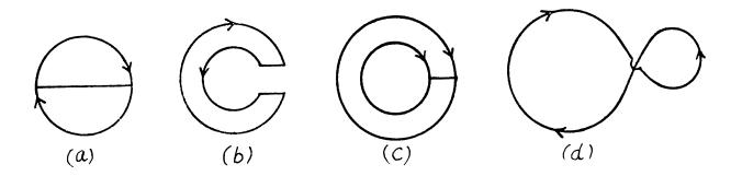
So, in figure (a), in the round conductor, it is clockwise and there is no current in the connector
