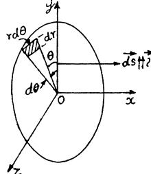
3.20 Let us consider an elemental surface area as shown in the figure. Then flux of the vector  $\overrightarrow{E}$  through the elemental area,
