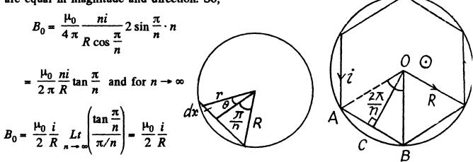
3.221 We know that magnetic induction due to a straight current carrying wire at any point, at a perpendicular distance from it is given by:
