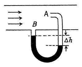
The gas flows over the tube past it at B. But at A the gas becomes stationary as the gas will move into the tube which already contains gas.
