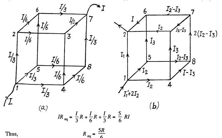
(b) Between 1 and 2 from the loop 14321,  $I_1 R = 2I_2 R + I_3 R$  or,  $I_1 = I_3 + 2I_2$
