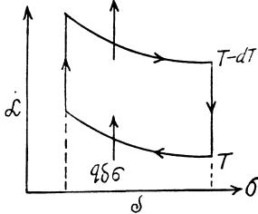
2.184 As before we can calculate the heat required. It, is taking into account two sides of the soap film
