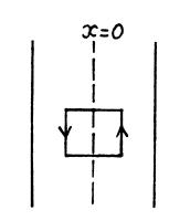
3.231 It is easy to convince oneself that both in the regions. 1 and 2, there can only be a circuital magnetic field (i.e. the component  $B_{\varphi}$ ). Any radial field in region 1 or any  $B_Z$  away from the current plane will imply a violation of Gauss' law of magnetostatics,  $B_{\varphi}$  must obviously be symmetrical about the straight wire. Then in 1,
