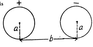
Note: if we require terms which depend on  $\frac{a}{b}$ , we have to take account of distribution of charge on the conductors.
