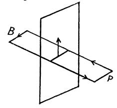
3.230 We assume that the current flows perpendicular to the plane of the paper, by circulation theorem,
