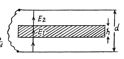
3.95 Given  $\overrightarrow{P} = \alpha \overrightarrow{r}$ , where  $\overrightarrow{r} =$  distance from the axis. The space density of charges is given by,  $\rho' = -\operatorname{div} \overrightarrow{P} = -2\alpha$
