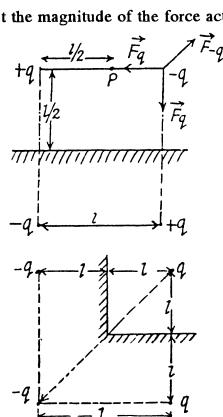
Using the concept of electrical image, force on the dipole  $\overrightarrow{p}$ ,
